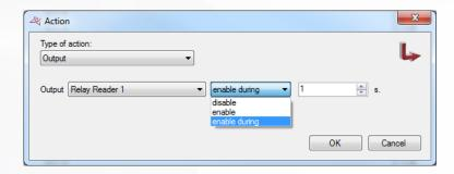
★ For an "External output" action, select a relay for a V-EXTIO module and then choose Enable, Disable, Invert or Enable during (1 to 65534 seconds).
