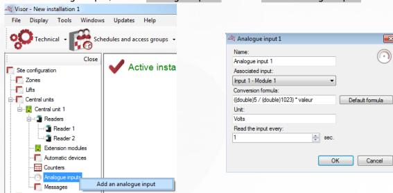
The analogue input is associated with a V-EXTIO module that first needs to be created in VISOR.
