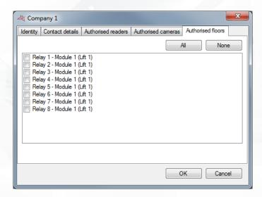
From this tab and in case of lifts, you can select for which floors the company has authorised access. This means that the company can only only affect these floors to its users.
