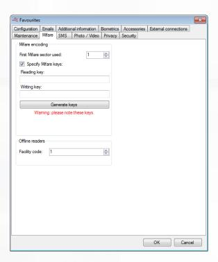
In this tab you can configure the encoding settings for the Mifare badges: you can then configure the index of the first sector that will be used, as well as the encryption keys.
