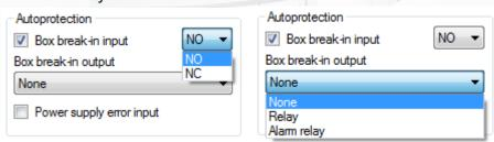
Check the "Power supply error input" box to generate an event if a failure occurs in the central unit's external power supply (a fault contact must be wired to the central unit). Select the type of contact (NO: normally open or NC: normally closed).
