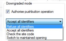
This mode becomes effective 30 seconds after a communication failure with the VERSO central unit.
