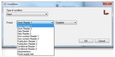
★ For an "External input" condition, select the input to be tested (only those in VEXTIO or VEXTLCD modules) and then select its status (enabled, disabled or sabotaged for the fourstate inputs of the VEXTIO modules).
