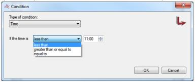
♣ For a "Date" condition, select the test method (if the current date is lower than / greater than / equal to) and then enter the date to be compared.
