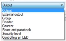
+ For an "Output" action, select one of the outputs of the Verso central unit and then choose Enable, Disable or Enable during (1 to 65534 seconds).
