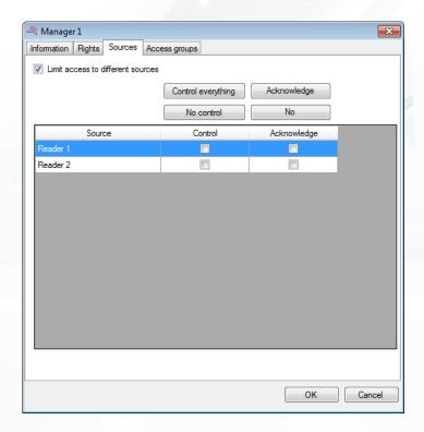
Check "Limit access to different readers" to filter the actions of this operator. For each reader, you can indicate:
