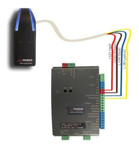
**NOTE:** If you are using an external power supply to power your proximity scanners, ensure that you connect all grounds to the ground on the control unit.
